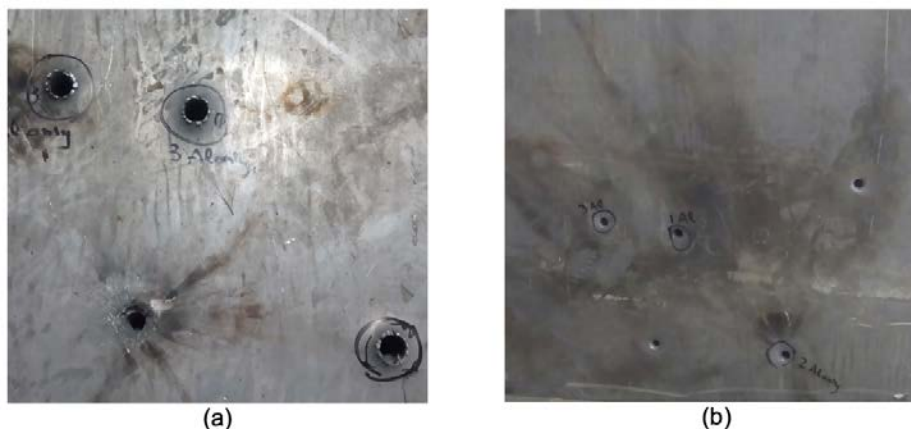
Figure 7: Holes caused by the penetration of the 12.7 mm AP tracer projectile in semi-infinite aluminium back plates (a) impact side of the first back plate (b) exit side of the second back plate.
