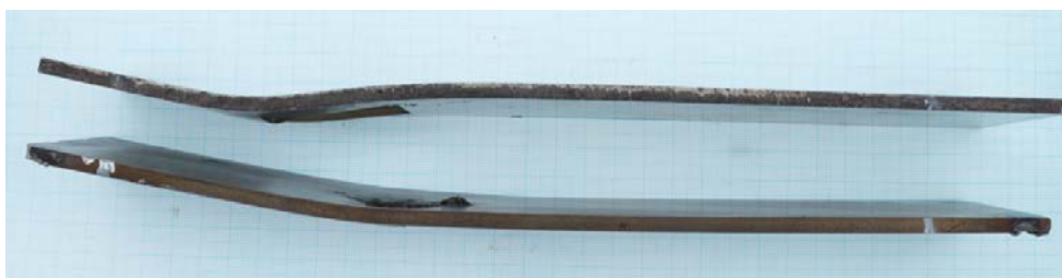
Figure 6: Target laminate after a shot: (a) entry hole – front plate face, (b) exit hole – front plate face, (c) perforated rubber – front face, (d) bent side steel plates (by an arrow the impact direction is indicated).
