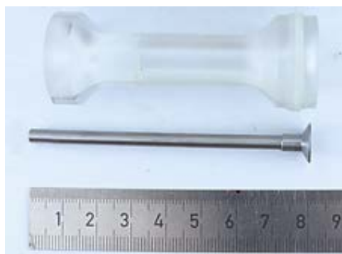
Figure 1: Down-scaled KEP with L/D = 20 and its sabot.
