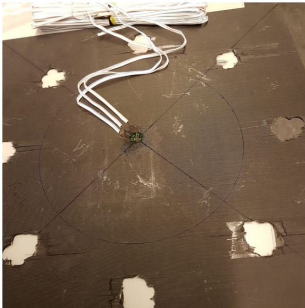
Figure 4: Rosette strain gauge attached at the back of the CFRP sample.
