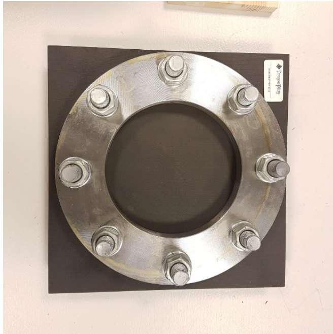
Figure 5: CFRP sample clamped in a circular flange of inner diameter 173 mm (top view).
