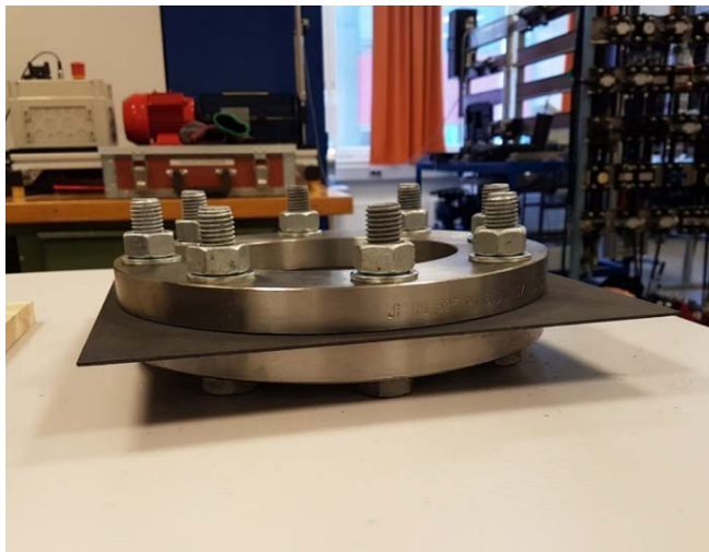
Figure 6: CFRP sample clamped in a circular flange (side view).
