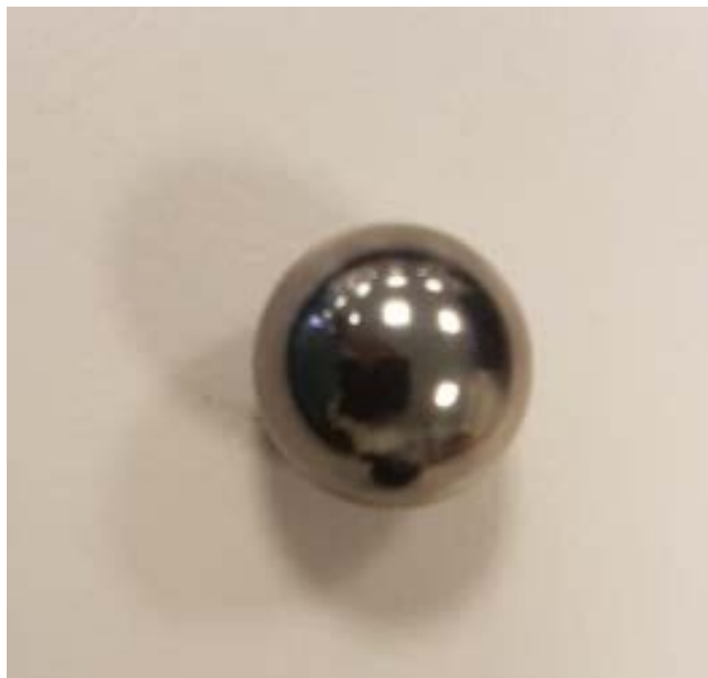
Figure 3: Steel ball (spherical) of 20 mm diameter and 33g weight.
