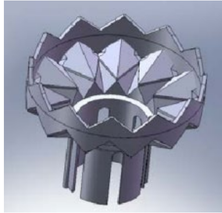
Figure 2. Structure of Settling Cup
