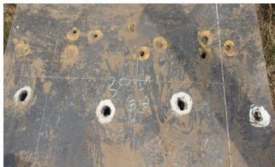
(b) Perforation of 30 mm target plate
