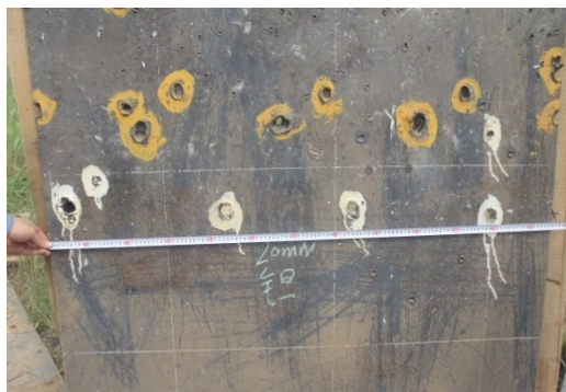
(a) Perforation of 20 mm target plate
